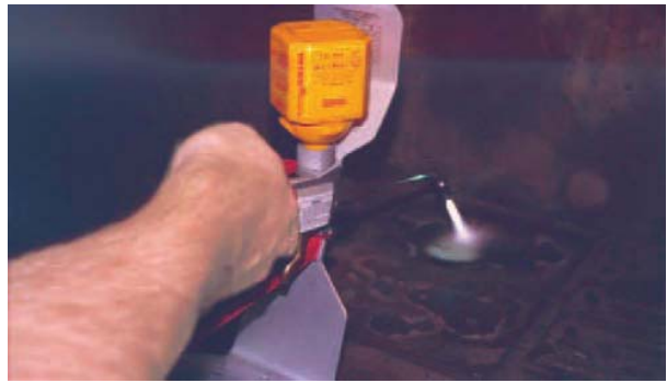
FIGURE 24-15 Rebuilding a worn crankshaft bearing with a Mogul Turbo-jet thermal spraying gun. Eutectic Corporation
