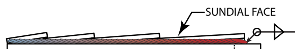
FIGURE 14-24 Small sealing weld on the outside edge of the sundial face. © Cengage Learning 2012
