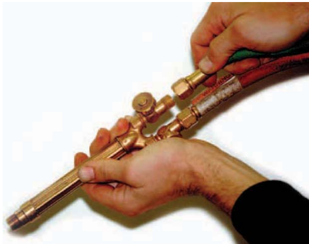
FIGURE 17-32 Connect the free ends of the oxygen (green) and the acetylene (red) hoses to the welding torch. Larry Jeffus
