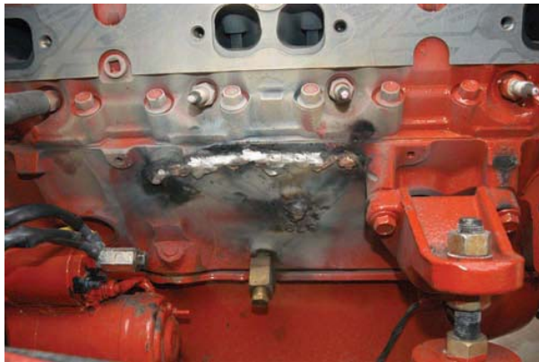
FIGURE 5-7D continued Grind the weld before finishing. Larry Jeffus
