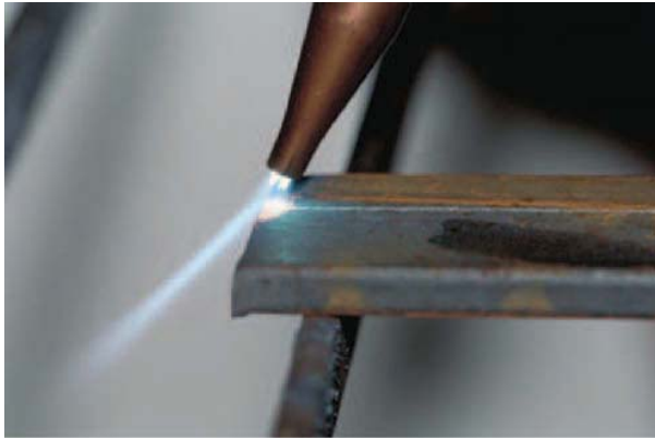
FIGURE 21-81 Beginning a cut with the torch concentrating the flame on the top edge to speed starting. Larry Jeffus
