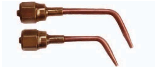
FIGURE 17-16 A variety of tip styles and sizes for one torch body. Larry Jeffus
