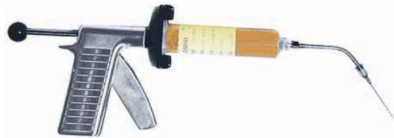
FIGURE 19-14 Gun for injecting flux into a joint Larry Jeffus
