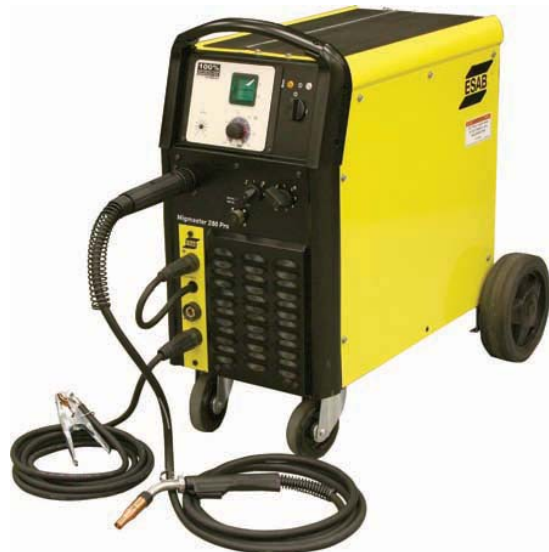
FIGURE 8-32 Power lug protection is provided by insulators. ESAB Welding & Cutting Products
