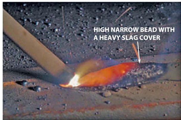
FIGURE 9-6 Welding with too short an arc length.
