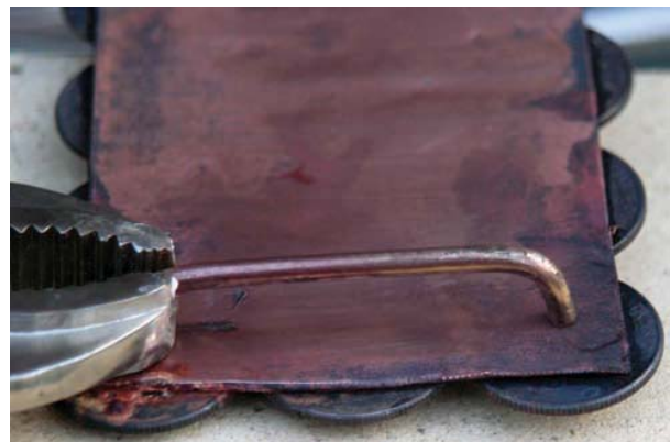
FIGURE 20-38 Use self-locking pliers to hold the belt loop in place. Larry Jeffus
