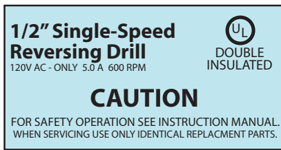
FIGURE 2-21 Typical portable power tool nameplate. © Cengage Learning 2012
