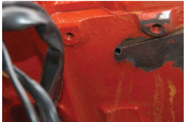
FIGURE 5-7B The drill hole will stop the crack from lengthening as it is being repaired. Larry Jeffus
