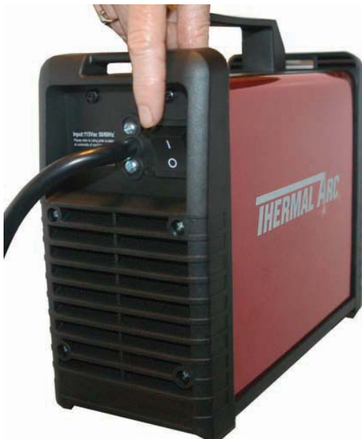
FIGURE 15-35 Always be sure that the power is off when making machine connections. Larry Jeffus
