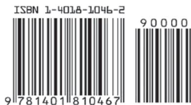
FIGURE 23-1 Bar codes are read by lasers to input information into computers. © Cengage Learning 2012
