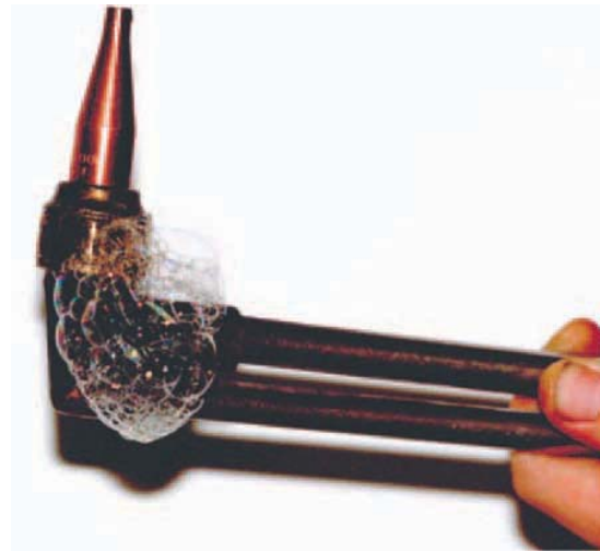
FIGURE 21-12 Checking a cutting tip for leaks. Larry Jeffus
