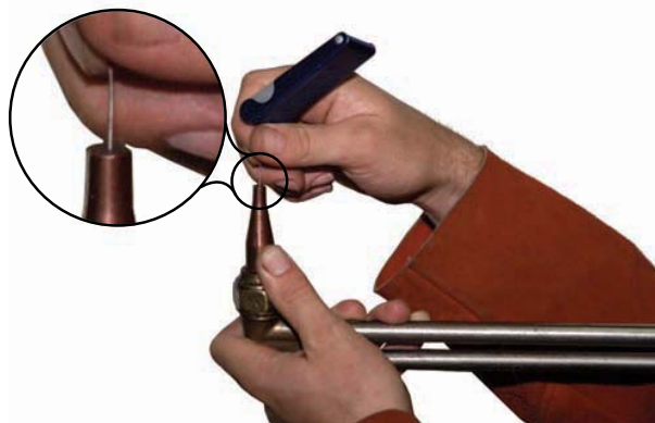
FIGURE 21-17 A tip cleaner should be used to clean the flame and center cutting holes. Larry Jeffus
