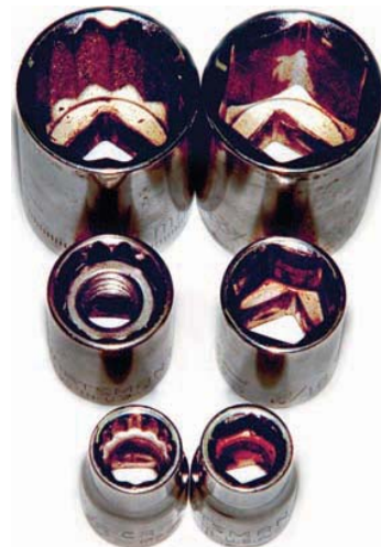
FIGURE 2-44 The fewer the points, the less likely the wrench is to slip. Larry Jeffus
