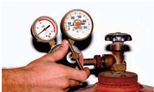
FIGURE 17-38 Adjust the regulator to read 5-psig working pressure. Larry Jeffus
