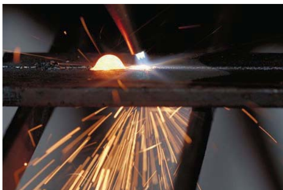
FIGURE 21-35 Poor cut. The slag is backing up because the cut is not going through the plate. Larry Jeffus
