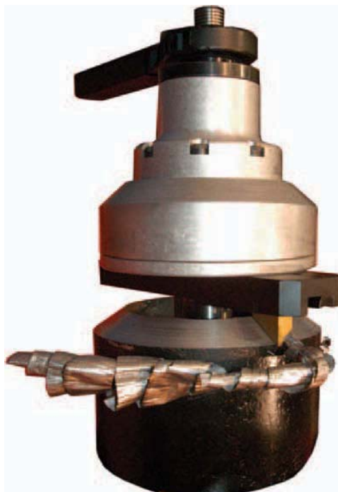
FIGURE 10-8 Pipe beveling machine. Larry Jeffus
