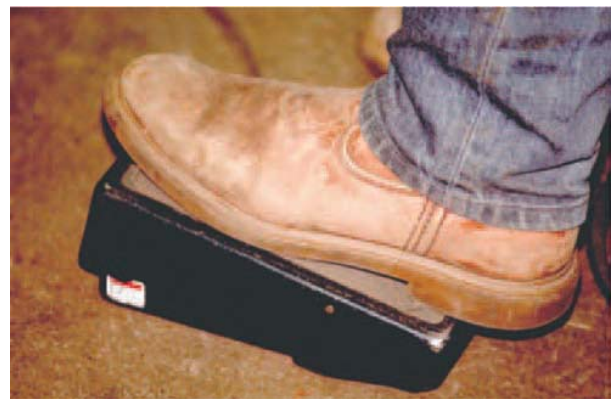
FIGURE 15-26 A foot-operated device can be used to increase the current. Larry Jeffus
