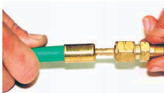
FIGURE 17-24 Screwing the hose nut onto a fitting will help when pushing the nipple into the hose. Larry Jeffus
