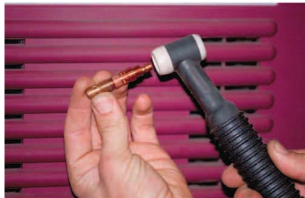
FIGURE 16-13 Inserting collet and collet body. Larry Jeffus
