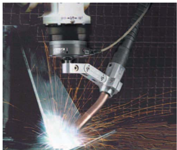
FIGURE 25-15 When using automatic equipment and robots, a break away collision sensor should be used. Applied Robotics, Inc.
