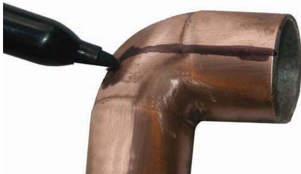
FIGURE 20-57 Marking a 90° to be cut for the corner piece. Larry Jeffus
