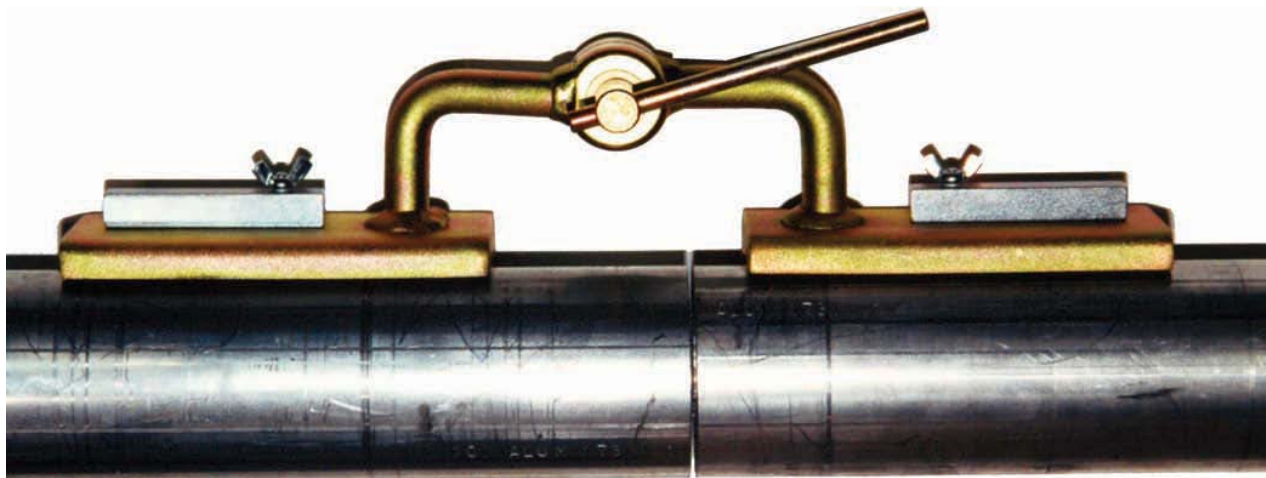
FIGURE 1-6 Magnetic alignment clamp used to hold pipe in the correct placement for welding. Larry Jeffus
