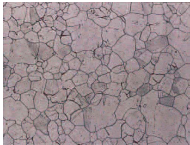
FIGURE 27-31 Microstructure of sensitized solution annealed type 304 stainless steel revealing austenite grain boundaries. George F. Vander Voort, Consultant
