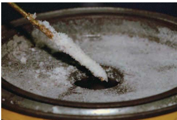
FIGURE 19-30C Flux stuck to rod ready for brazing. Larry Jeffus
