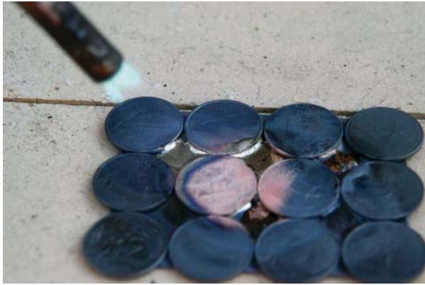
FIGURE 20-32 Filler metal flowing under the coins. Larry Jeffus
