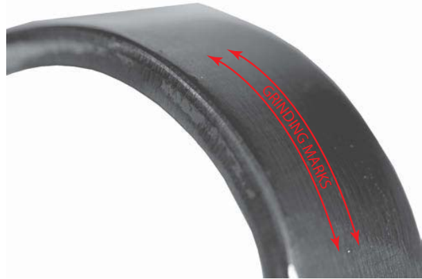
FIGURE 29-6 Guided-bend tested specimen. Larry Jeffus
