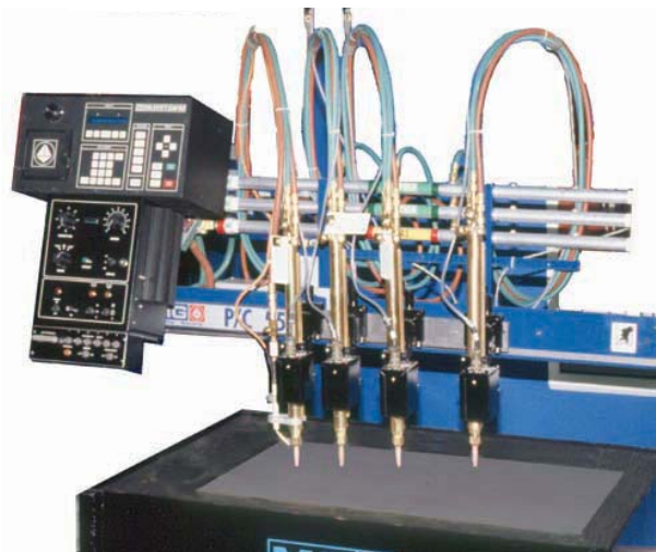
FIGURE 7-8 Four cutting head automatic flame-cutting machine. Larry Jeffus
