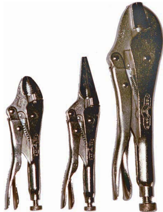
FIGURE 6-46 Three common jaw types on locking pliers. Strong Hand Tools & Good Hand, Inc.
