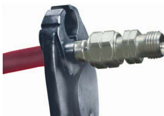
FIGURE 17-25 Crimping hose ferrule. Larry Jeffus
