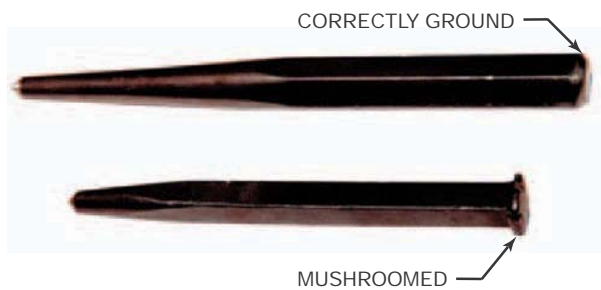
FIGURE 2-45 Any mushroomed heads must be ground off. Larry Jeffus
