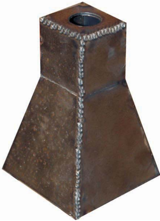
FIGURE 20-6 Candlestick from Project 21-2 can be decorated with a braze covering. Larry Jeffus
