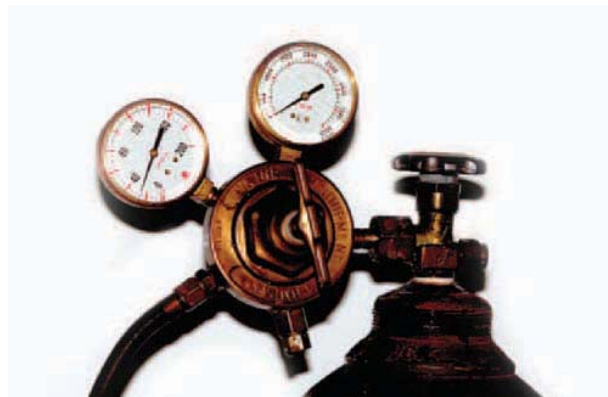
FIGURE 17-34 Back out both regulator adjusting screws before opening the cylinder valve. Larry Jeffus
