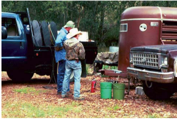
FIGURE 21-25 Have plenty of water and a fire extinguisher available before starting to cut or weld. Larry Jeffus
