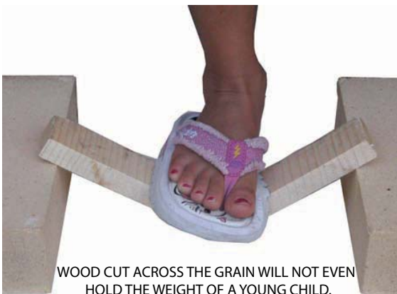
FIGURE 21-76 Metal, like wood, is stronger with the grain than it is across the grain. Larry Jeffus
