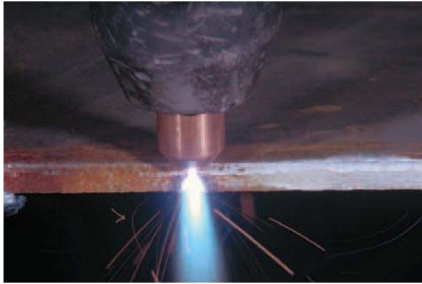
FIGURE 22-31 The spark stream should be blowing the metal away from the bottom of the plate. Larry Jeffus
