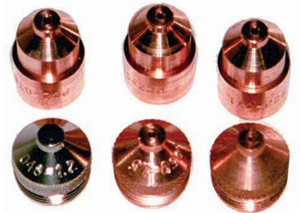
FIGURE 22-7 Different torches use different types of nozzle tips. Larry Jeffus
