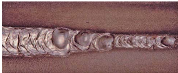
FIGURE 10-15 Uniformity in each pass shows a high degree of welder skill and increases the probability that the weld will pass testing. Larry Jeffus
