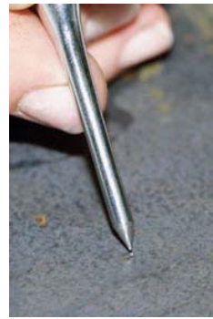
FIGURE 18-23 Center punching the plate for drilling. Larry Jeffus
