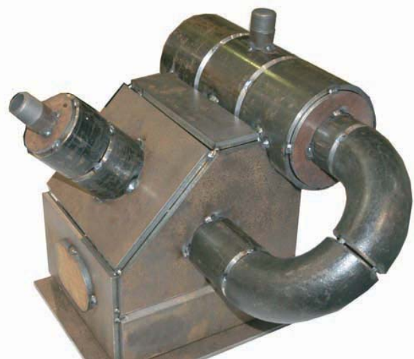
FIGURE 6-39 Welded assembly fabricated at SkillsUSA competition. Larry Jeffus
