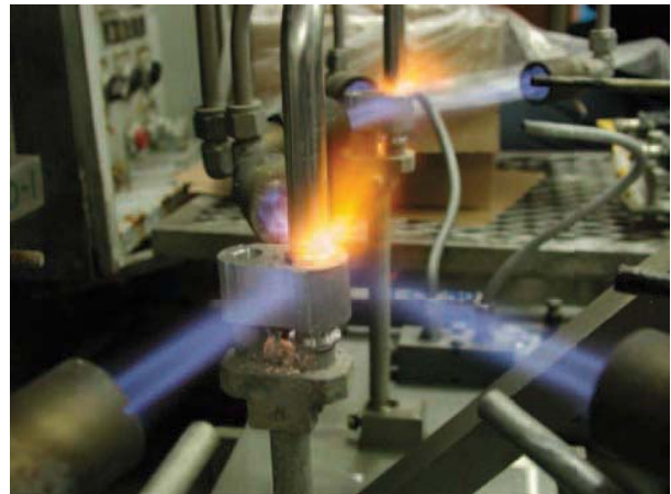
FIGURE 25-14 Rotating worktable increases the work zone. Eutectic Corporation
