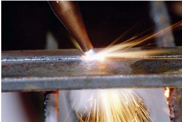
FIGURE 21-49 The torch is rotated to allow the preheating of the plate ahead of the cut. This speeds the cutting and also provides better visibility of the line being cut. Larry Jeffus
