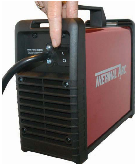
FIGURE 16-6 Always be sure the power is off when making machine connections. Larry Jeffus
