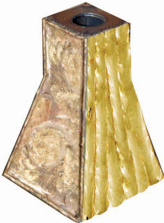
FIGURE 20-7 Two ways of finishing the brazed surface. Larry Jeffus
