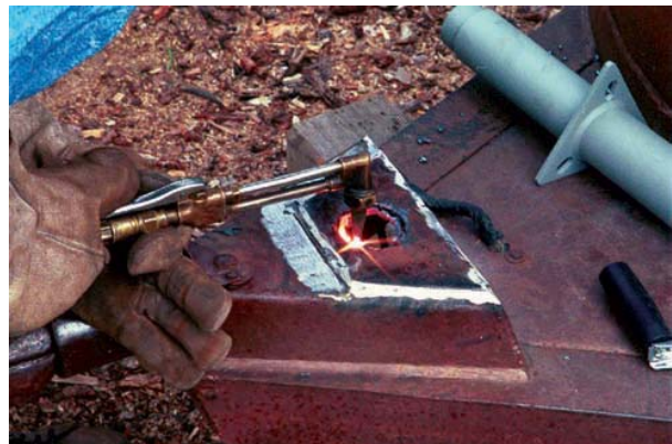
FIGURE 21-27 Bracing your hand on the tractor tongue will help keep you steady as you make the cut. Larry Jeffus
