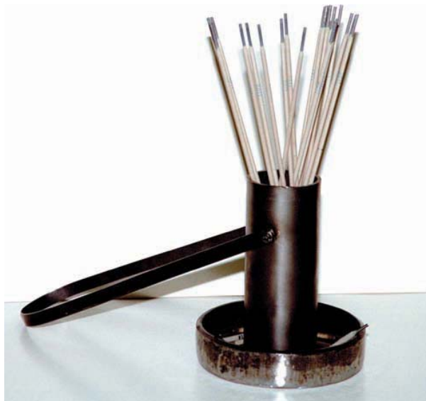
FIGURE 2-42 An easy-to-build electrode caddy can be used to hold both electrodes and stubs. Larry Jeffus
