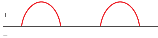
FIGURE 8-28 One rectifier in a welding power supply results in pulsing power. © Cengage Learning 2012
