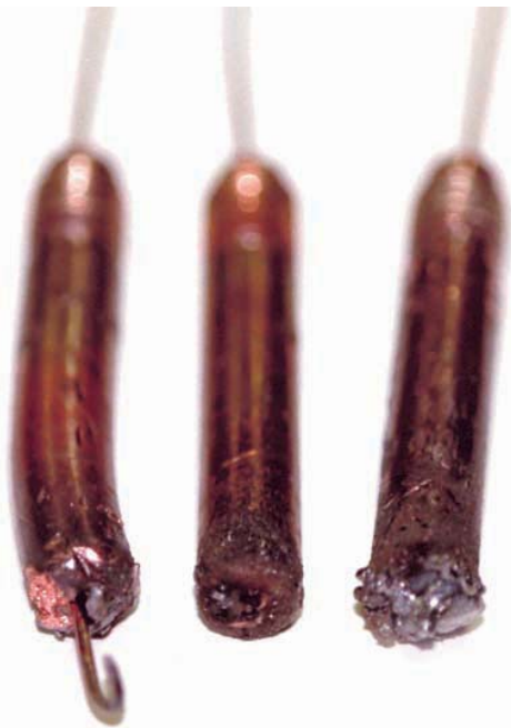
FIGURE 11-7 Excessive heat can damage the contact tube. Larry Jeffus
