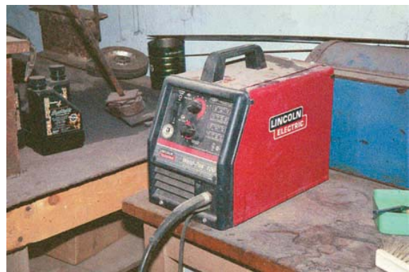
FIGURE 13-31 FCA welders can be small and durable enough to be used where SMA welders once dominated. Larry Jeffus
