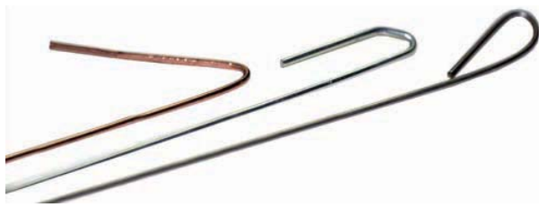
FIGURE 18-11 The end of the filler rod should be bent for safety and easy identification. Larry Jeffus
