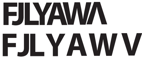
FIGURE 16-47 Nesting the parts can save material. © Cengage Learning 2012
