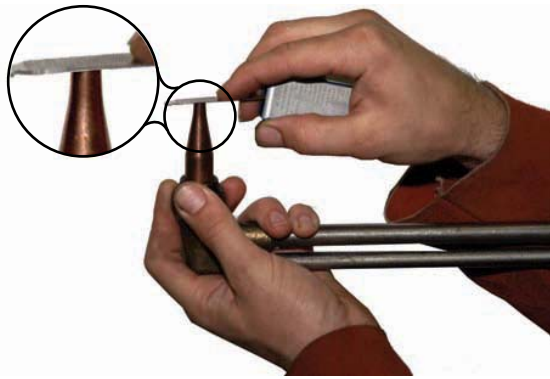
FIGURE 21-16 File the end of the tip flat. Larry Jeffus
