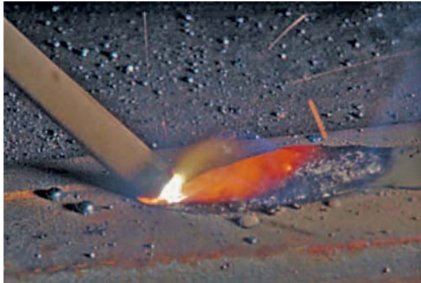
FIGURE 9-35 Making the weld narrow with a higher buildup by using a short arc length can add dimension to the finished project's surface appearance. Larry Jeffus
