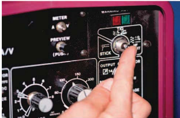
FIGURE 16-11 The high-frequency switch should be placed in the appropriate position. Larry Jeffus
