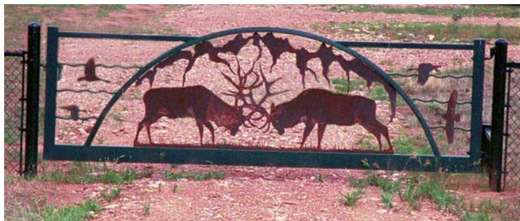
FIGURE 22-2 Plasma-cut sheet metal panels decorate this gate. Larry Jeffus
