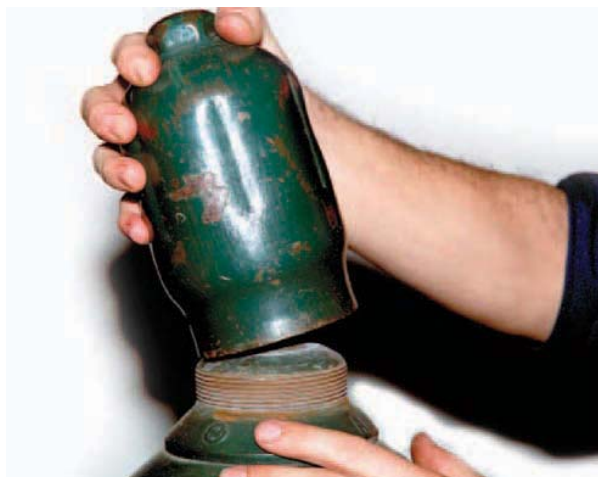
FIGURE 17-27 Unscrew the valve protector caps. Put the caps in a safe place as they must be replaced on empty cylinders before they are returned. Larry Jeffus
