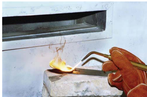
FIGURE 2-16 Flexible exhaust pickup. Larry Jeffus
