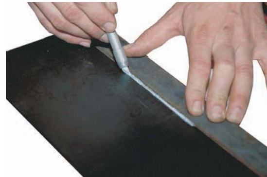
FIGURE 6-33 Make sure that the soapstone is held tightly into the part being traced. Larry Jeffus
