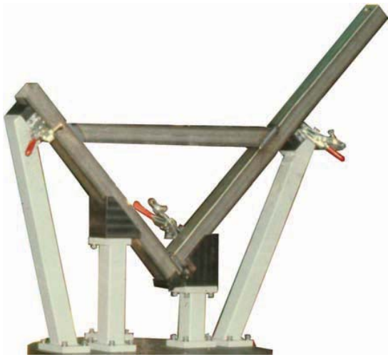
FIGURE 7-1 Welding jig used to hold square tubing in alignment for welding. Larry Jeffus
