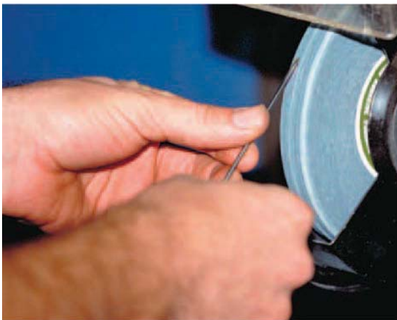
FIGURE 15-27 Correct method of grinding a tungsten electrode. Larry Jeffus
