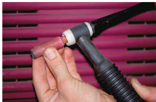
FIGURE 16-14 Install the nozzle (cup) to the torch body. Larry Jeffus
