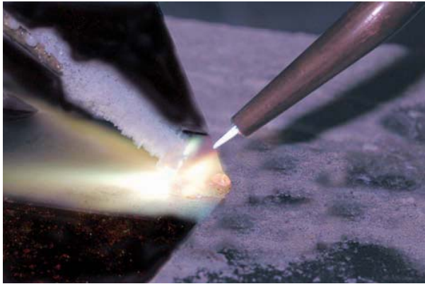
FIGURE 20-8 Heating the metal to make a tack braze. Larry Jeffus
