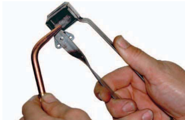
FIGURE 17-41 Correct position to hold a spark lighter. Larry Jeffus
