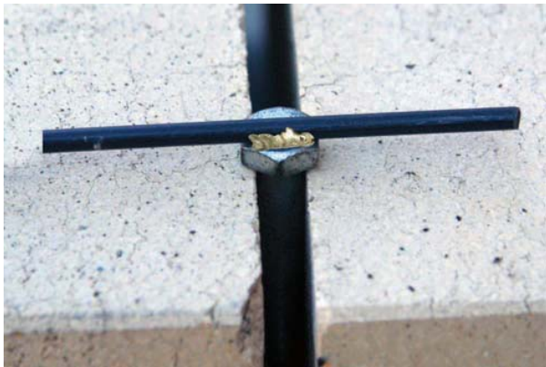
FIGURE 20-16B Braze the T handle to bolt head. Larry Jeffus
