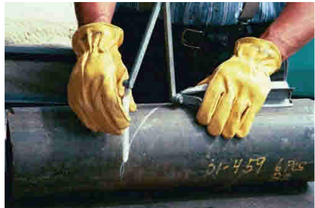
FIGURE 21-89 The flexible arms allow a mark to be drawn completely around the pipe. Larry Jeffus
