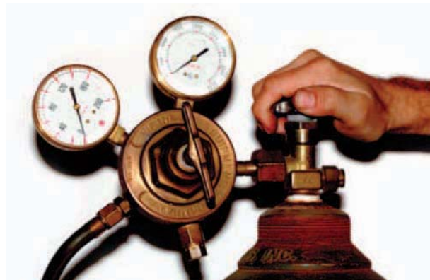
FIGURE 17-35 Stand to one side when opening the cylinder valve. Larry Jeffus
