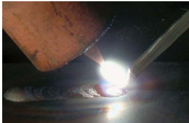
FIGURE 16-29C Dipping the filler metal at a constant rate will keep the weld bead produced uniform. Larry Jeffus
