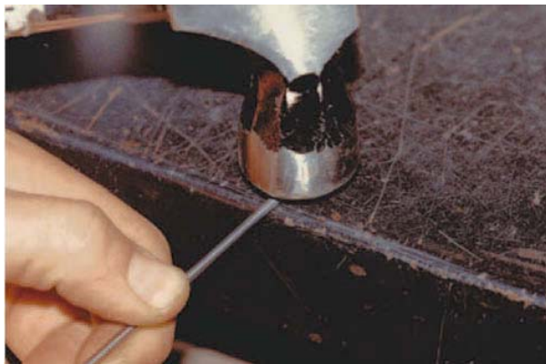
FIGURE 15-30 Breaking the contaminated end from a tungsten by striking it with a hammer. Larry Jeffus
