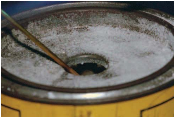
FIGURE 19-30B Dipping the heated rod into the flux. Larry Jeffus
