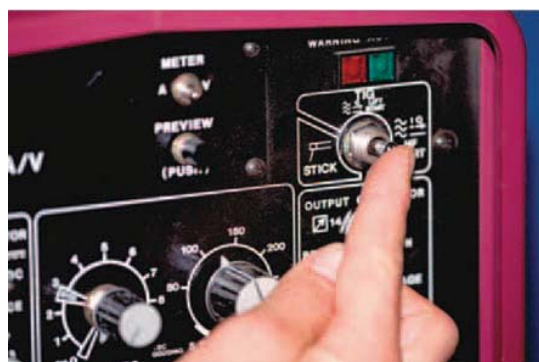
FIGURE 15-40 The high-frequency switch should be placed in the appropriate position. Larry Jeffus
